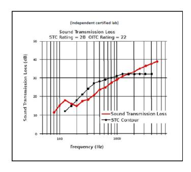
**Sound Transmission Loss Test Results**
